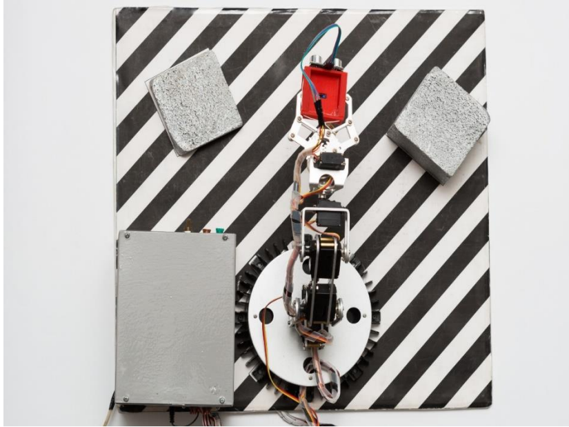
Fig. 1. The Robotic Arm as an actuator of color sorting objects system.
